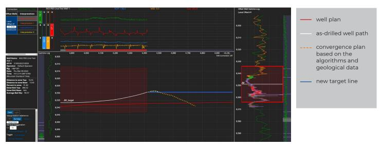
Drilling geology integration enables an early target change, avoiding an unnecessary slide.
