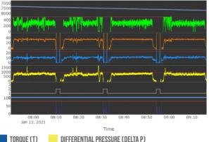
> Higher differential pressure maintained with the Autodriller<sup>®</sup> Pro control system—contributing to higher ROP
