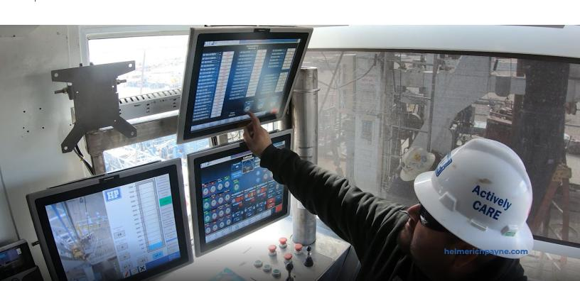
In this case, where the team suspected a weak motor, H&P lowered the StallAssist software setpoints to try and detect a stall sooner and prevent the motor from reaching the maximum stall PSI rating, helping to extend the life of the weak motor.
